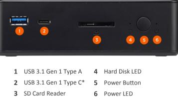
\*NC10U3/U5/U7 with Intel Core processor supports USB 3.1 Gen 2 (Type A and C)
